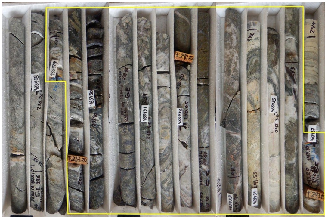
Hole No. 526010: Viridiana vein (236.90 – 243.35 m; 6.45 m). Arista System Q1 2026. 5.6 m estimated true width at 7.97 g/t AuEq of $1,113/t NSR (0.49 g/t Au, 442 g/t Ag, 0.21% Cu, 5.27% Pb, 13.86% Zn)
