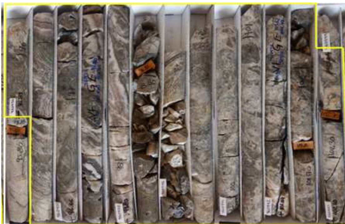
Hole No. 525061: Marena North vein (95.83 – 102.58 m; 6.75 m). Arista System Q3 2025. 5.23 m estimated true width at 5.06 g/t AuEq of $450/t NSR (3.21 g/t Au, 169 g/t Ag, 0.40% Cu, 2.88% Pb, 4.92% Zn)
