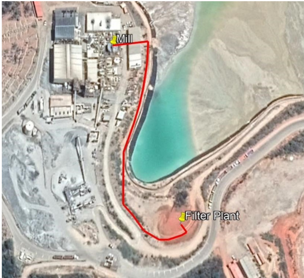
Figure 10-4: Pipeline Route for Filtered Tailings Feed Pipeline.
