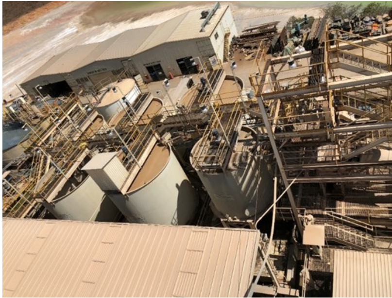
Figure 14-5: Agitated Leach Circuit of the DDGM Processing Facility.
