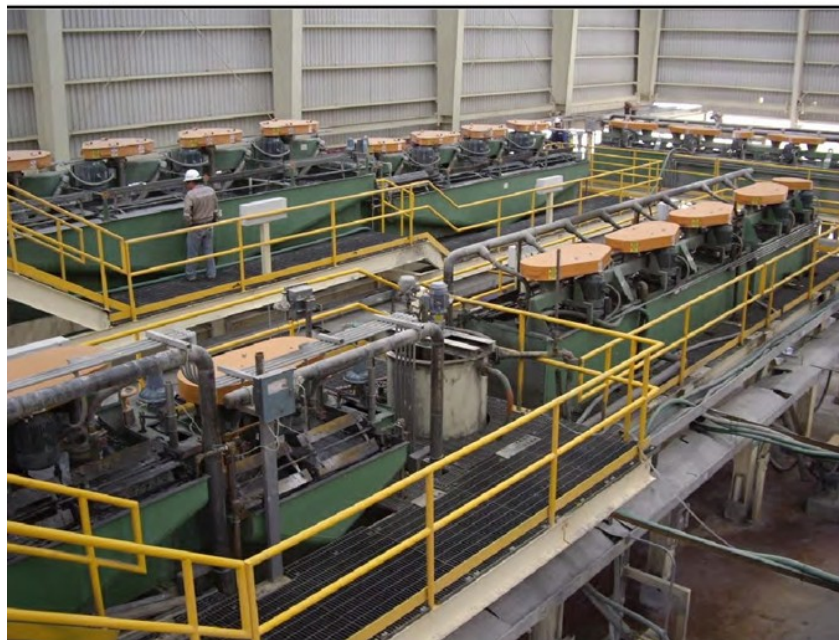
Figure 14-4: Banks of Flotation Cells at the DDGM Processing Facility.
