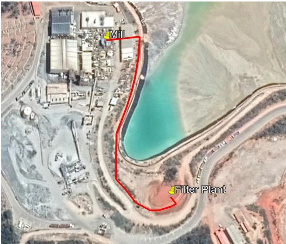
Figure 10.4 Pipeline Route from Filter Plant to Paste Plant
